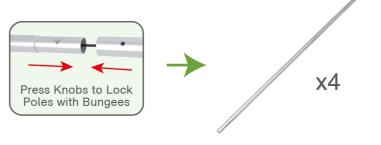
**STEP 02** Connect long poles with corner poles according to labelings.
